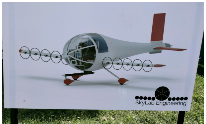
Many aircraft designs capitalize on the "Blown Wing" concept and fueled engines generating power for electric wing mounted motors.
