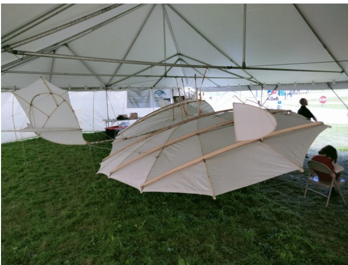
In 1896 Otto Lilienthal designed and flew his Vor-flugelapparat glider. Note the similarities to today's aircraft that use winglets, and leading edge slats.
