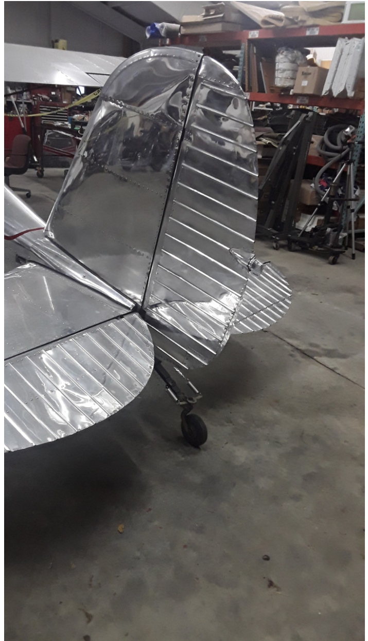
ADS-B (Uvionx) works from tail light position! (yes, new tail springs/chain, etc)
