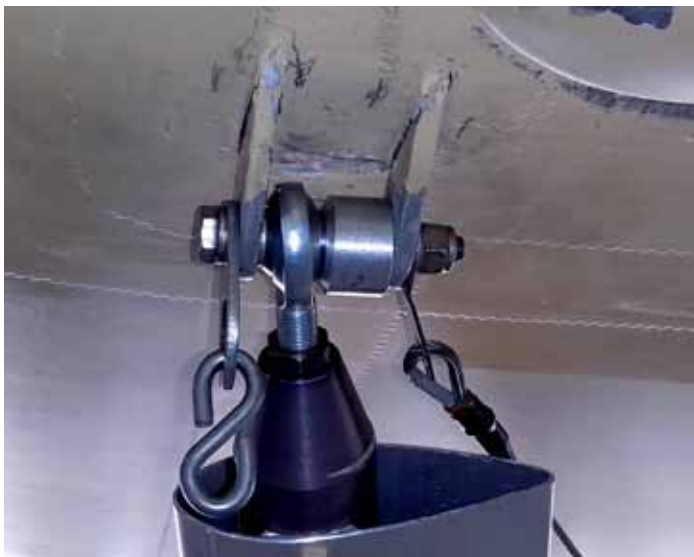
Completed front strut bracket assembly. The diagonal brace wire has yet to be tightened. The spherical spacer
