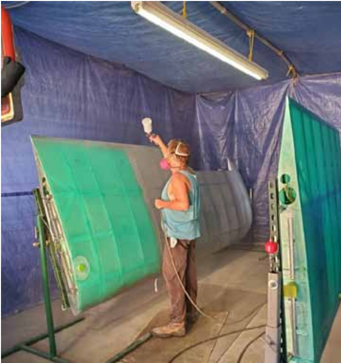
1946 Cessna 120 wings being painted, Ceconite fabric with silver coating.
