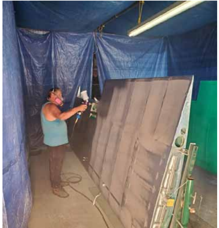
Below: Finished wings with several coats added for UV resistance.
