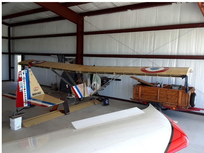
Ailerons are removed for inspecting the aft spar and lubricating the aileron pivot points.
