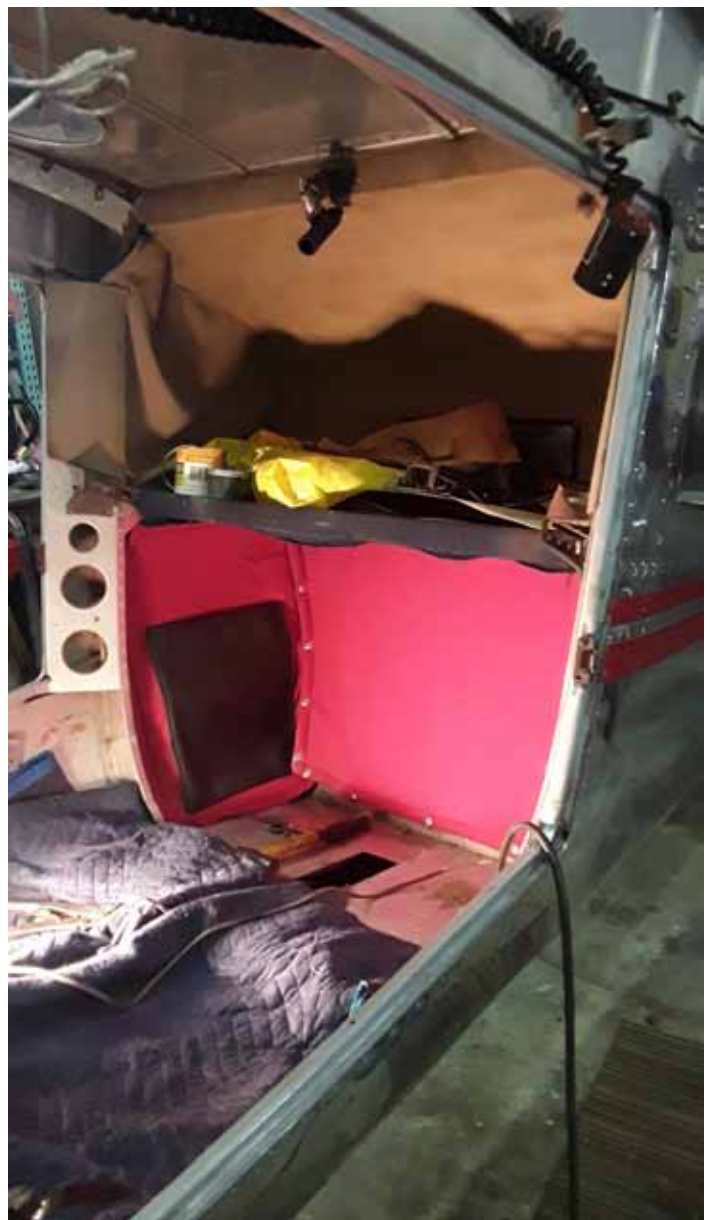
Another interior photo, with seat removed to access space below the unfinished "hat rack" but, a new, red, silencing pad reinstalled just in front of battery and it's box.
