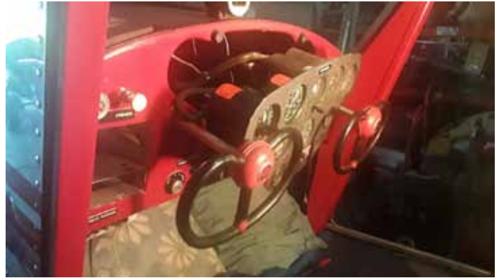
Reinstall instrument panel with a few reconditioned/tagged instruments.
